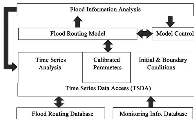
**Fig. 2.** Schematic layout of the flood system framework
